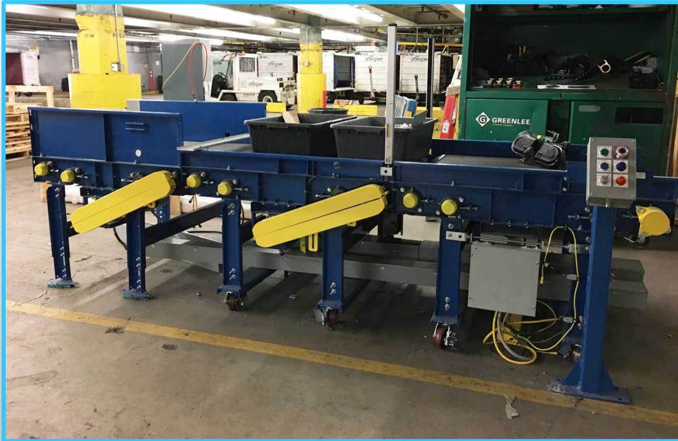
BHS conveyor mock-up under review
